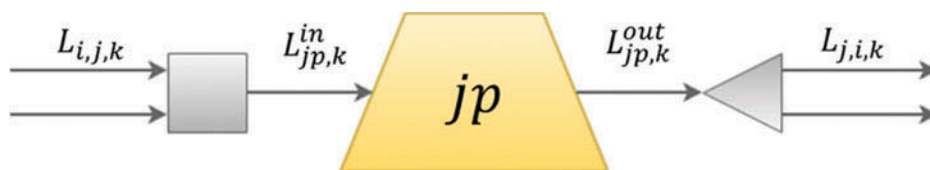
Figure 1. Generic superstructure of streams considered in one heap system. L_{jp,k}^{in} and L_{jp,k}^{out} represent the input and output mass of the k species in the heap jp . L_{i,j,k} and L_{j,i,k} correspond to the flows before and after the virtual mixing and splitting units, respectively.
